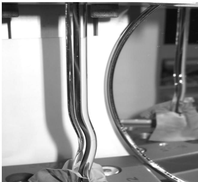
Fig. 3. A helically buckled filament (white) is visible inside a glass tube filled with blue dye. Regions where the filament touches the wall can be distinguished by its white appearance given a minimal amount of blue dye that exists between the filament and wall at points of contact.
